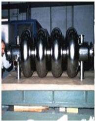
Superconducting LEP cavity
